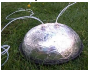
Figure 2. Non-transparent chamber with compensation tube
