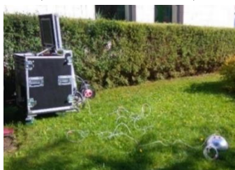
Figure 1. Chamber connect with Picarro G2508
