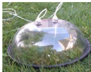
Figure 3. Transparent chamber with compensation tube
