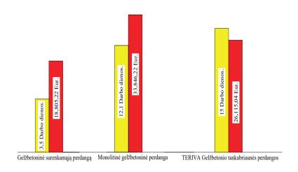
with the least amount of time and money costs, according to the comparison. It would take 12.1 working days to complete the monolithic reinforced concrete overlay, which costs 33,846 EUR. This price includes two layers of reinforcement work with reinforcement. The longest number of working days would be required to install the Teriva reinforced concrete tank rib overlay.
